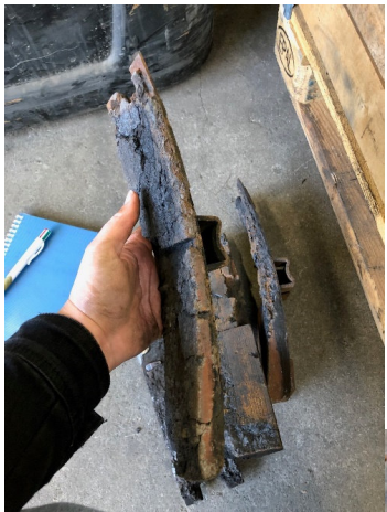
All IB116* after unintended brake applications
